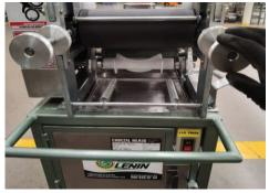
Adjust the gordita thickness by turning the adjustment knobs (clockwise to make the tortilla thinner, and counterclockwise to make it thicker) Lower the clutch lever when you obtain the desired thickness
