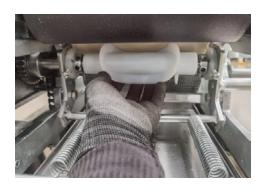
Place the cutter on the base, and verify that it is correctly installed and secured
